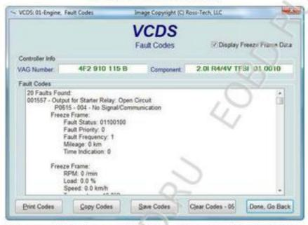
On this screen, VCDS shows you any DTCs ("Diagnostic Trouble Codes" or Fault Codes) present in the control module in which a communications session is currently active. VCDS shows the DTC numbers and also decodes each DTC into meaningful text.
