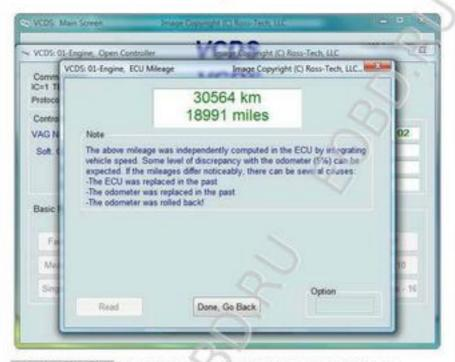
[EDC-15-16 Mileage] is found in the Applications Screen and is used to show an independent "odometer" reading stored in the ECU. EDC-15 is found in older TDI engines like the North American market VE 1.9L Golf/Jetta/etc. EDC-16 is used in 2.0L TDI's including all North American PD engines, but not in the newest CR engines. This function can be useful as a means of cross-checking the mileage on a used car before making a purchase, particularly in Europe where odometer fraud is rampant.
