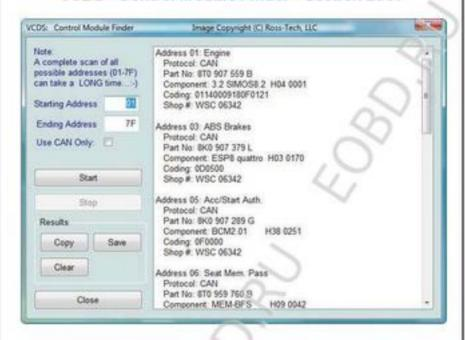
This function cycles through each possible address in the vehicle, finding each controller and reporting its Address, Name, Protocol, VAG Number, Component Number, Soft. Coding, and WorkShop Code.
