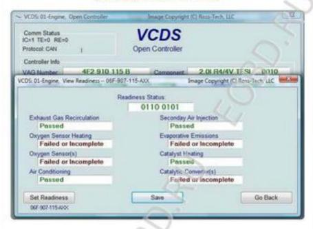
The Readiness Code is a set of 8 bits, each of which corresponds to one monitored emissions "system" in an OBD-II car. When all readiness bits show "Passed", it means that all systems have been checked and have passed the on-board tests. The Readiness screen shows name of script in tide bar and under the [Set Readiness] button, or gives a reason why [Set Readiness] is disabled when that is the case.
