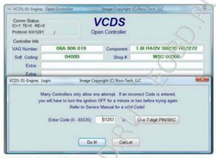
The Login Function must be used on some (but not all) Control Modules before you can Recode or change Adaptation values. On others, it "enables" certain features like cruise control. Valid Login codes can be found in the Factory Repair Manual for your car.
