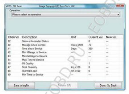
Models using flexible service intervals may show "---" as values for the time/distance to the next service in the instrument cluster. This is not an error. The system requires a certain time/distance to calibrate itself to show meaningful values, usually this takes about 300 miles or 500 km:
