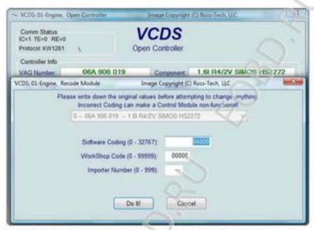
Recode is used to set various options in a Control Module. Note: Some Modules require a valid Login before you can re-code them.
