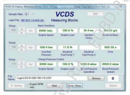
Export RPM Only when checked will record only RPM from the first field and will not record other fields. Also, this will only record RPM values that are non-zero. This feature can be useful if you are logging to cutput the file to a spreadsheet or other third party software.
