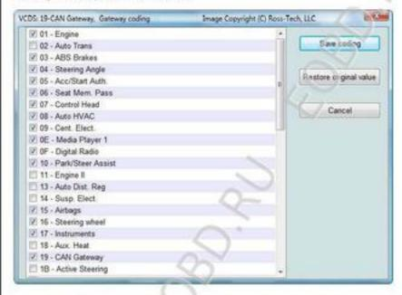
Use the [Do ItI] button to save the new Soft Coding to the controller and return to the Open Controller Function screen.
