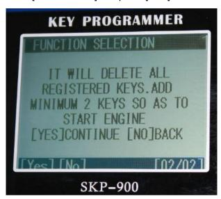
As shown on the screen, you must add at least 2 new keys to start the engine after deleting all registered keys.
