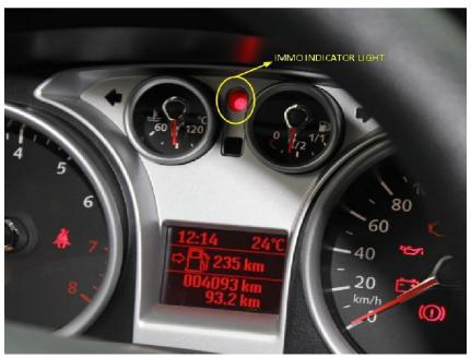
According to the instruction on screen, you should insert a new key and turn IGN on. You may see the IMMO indicator light will flash when inserting a key which cannot start Engine.
